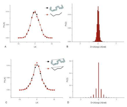
Fig. 3. Figure A shows the normalized probability distribution of LK for the original and the corresponding reduced chains in a PE-1000 melt and Figure B the probability distribution of the corresponding differences. Figure C shows the normalized probability distribution of LK for the original and reduced chains after end-to-end closure and Figure D shows the corresponding differences
