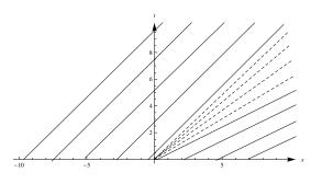
Figure 3.3: Characteristic lines illustrating rarefaction.
