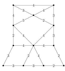
**Solution:** Kruskal's algorithm begins by selecting a minimum weighted edge. We have 5 choices for an edge of weight 2. Here, we pick the edge on the left hand side.
