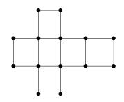
**Solution:** An Eulerian circuit is a closed trail that contains each edge of a graph. We saw in class that a connected graph is Eulerian if, and only if, each vertex has even degree. The vertices indicated below both have degree 3, which is odd. Hence, the graph cannot be Eulerian.
